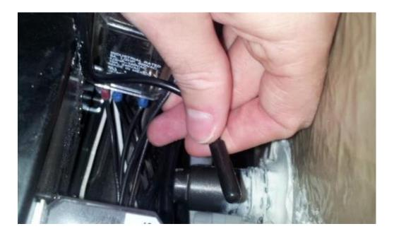
Connect the three computer control box wires on top of the Royal Spa control box. Match wires labeled FLOAT, 12V, and SOUND to their corresponding labels. The metal forks are tightened down underneath each corresponding screw on the control box. (Float, 12V, Sound)
