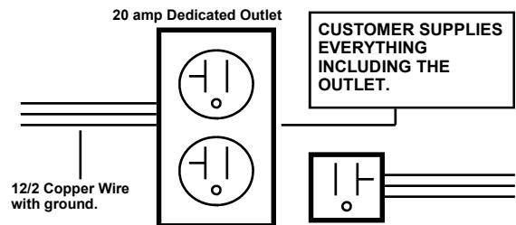
**NO EXTENTION CORDS** are to be used in conjunction with the operation of the spa. Low voltage damage could result which is not covered by warranty. All electrical work must be done according to NEC (National Electric Code) and any other applicable electrical codes.
