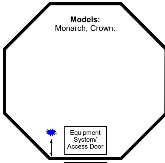
For wiring a “Crown” or “Monarch”, start at the corner immediately to the left of the Access Door. From that corner, measure **12 inches** back from the Access Door wall. This location is the best stub-up location for your electrical connection.
